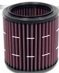
4.5" OD x 3.3" ID 4.8' high and sliced twice at white lines
