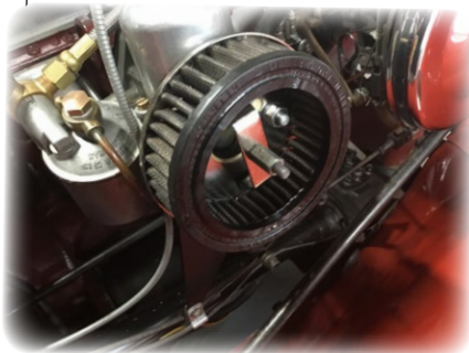
4.5" OD x 3.3" ID 4.8' high and sliced twice at white lines
