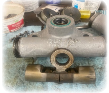
Support the body and press out the shaft.
