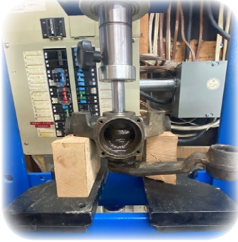
Support the body and press out the shaft.
