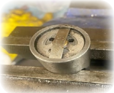
Views of the end of the piston showing the orifices which control the flow of oil through the piston body.
