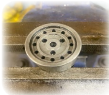
Views of the end of the piston showing the orifices which control the flow of oil through the piston body.
